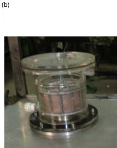
Fig. 1. Schematic of the impinging stream–rotating packed bed unit. (a) Schematic diagram of the IS-RPB; (b) digital photo of the IS-RPB.
